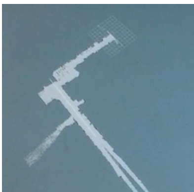
Figure: 23: Mapping - 2-Dimensional map created in rviz software using hector mapping as the robot navigates to the destination.
