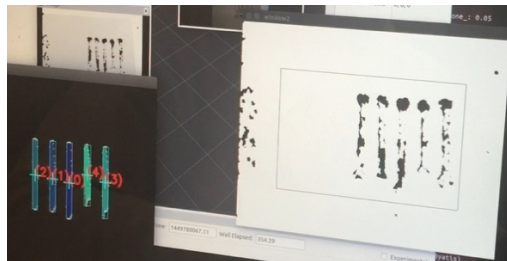
Figure: 25: Wrench detection - The above picture shows the wrench detection package run on the client computer. The smallest wrench is shown with the largest number on the left window. Therefore, we can conclude that the smallest wrench is the second wrench from the right in the above case.
