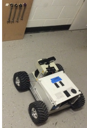
Figure: 24: Wrench Detection - Robot is positioned to detect the smallest wrench on the board.
