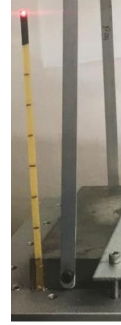
Figure 4: (a) Experimental FRFs of fettuccine strands of varying lengths (Input: acceleration of the base, Output: Tip-velocity of the fettuccine strand), (b) Dynamic test of a single cantilevered fettuccine strand
